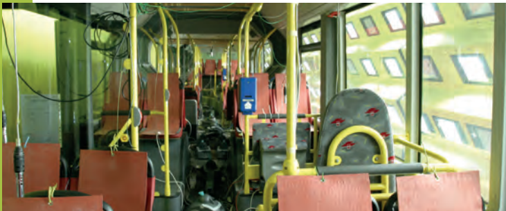
Fig. 1: heating mats simulate passengers
