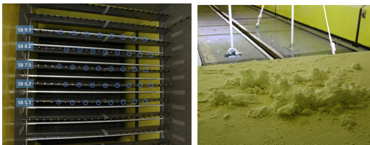
Figure 27: Nozzle setup for blowing snow tests in the RTA IWT and snow piled up
