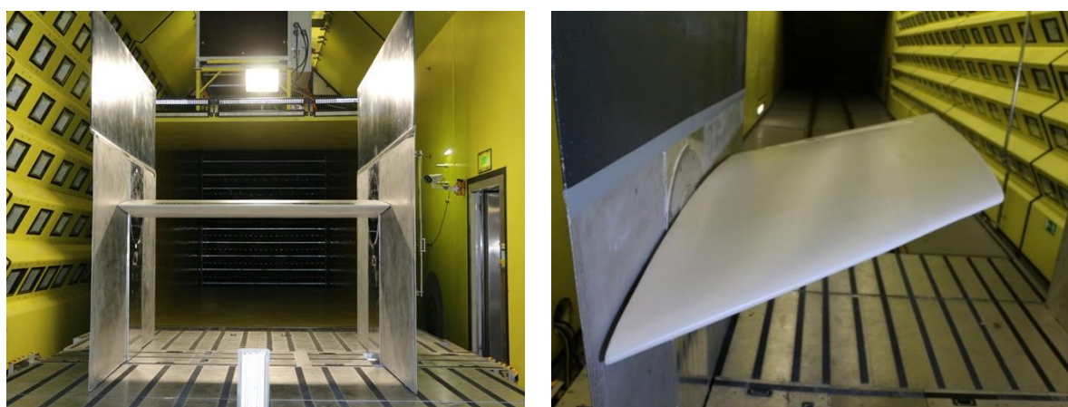
Figure 19: Test setup for a wing section test inside the IWT
