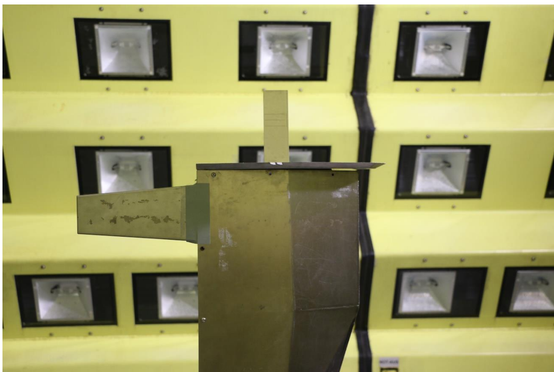
Figure 43: Automatic icing blade installed in the test section
