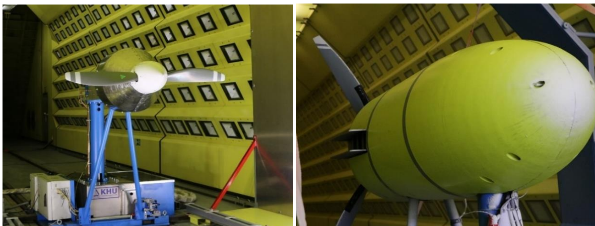
Figure 25: Standard configuration of the prop Rig shown in the left image. A cover can be used for the rear part of the test bench for the pusher configuration as shown in the right image.
