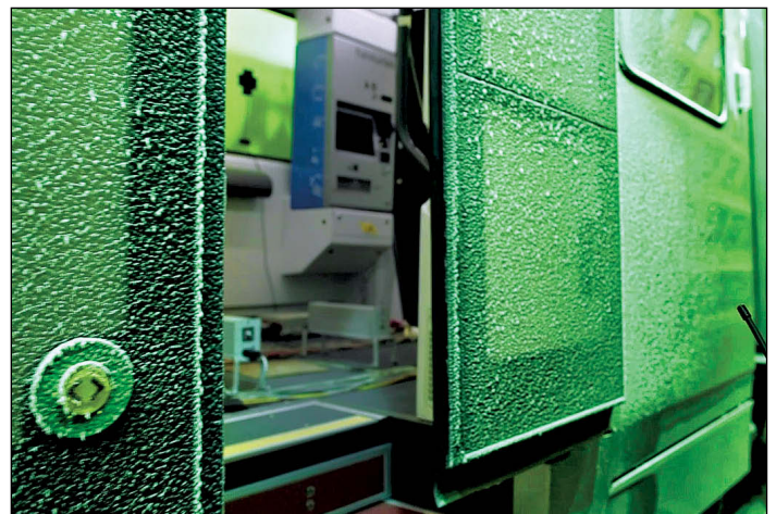
Figure 2: Example of door opening test.
