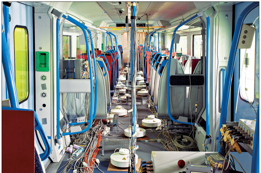
Figure 5: Typical test set-up with passenger load simulation in a rail vehicle.
