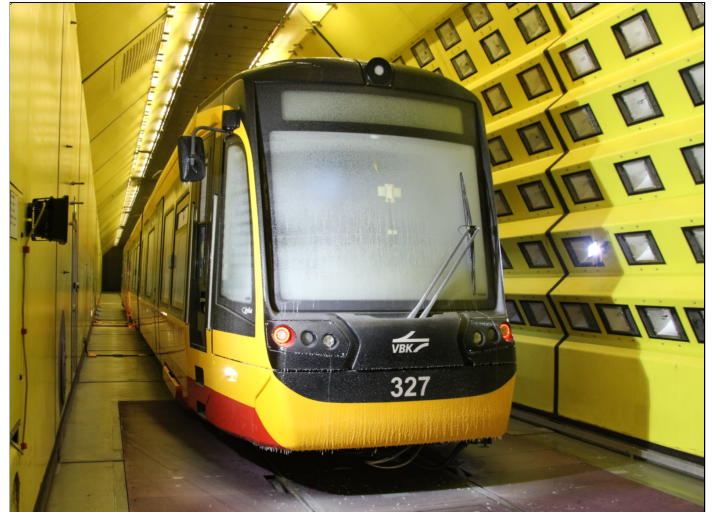
Photo 1: Vehicle prepared with ice layer for function tests (testing of Tram-Train Karlsruhe).
