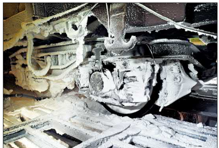
Photos 4: Test setup with freight waggon for brake block winter certification tests.
