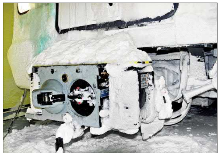
Photo 5: Testing the effectiveness of the coupling heater under snow conditions.
