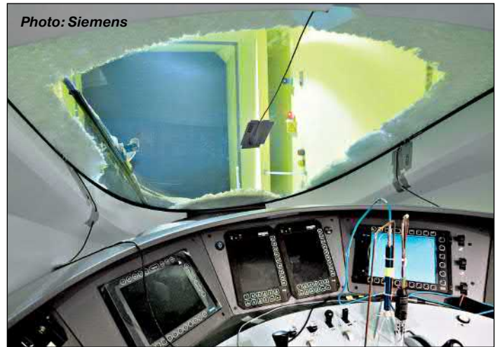
Photos 6: Defrosting of wind screen for driver visibility (testing of a DB's Class 407 Velaro high speed train).
