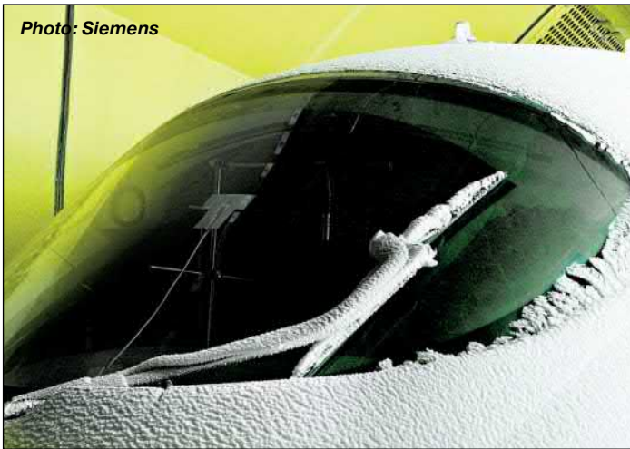
Photos 6: Defrosting of wind screen for driver visibility (testing of a DB's Class 407 Velaro high speed train).
