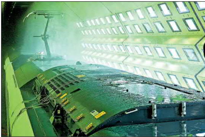
Photo 2: Water tightness test of roof components.
