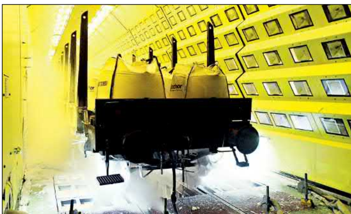
Photos 4: Test setup with freight waggon for brake block winter certification tests.
