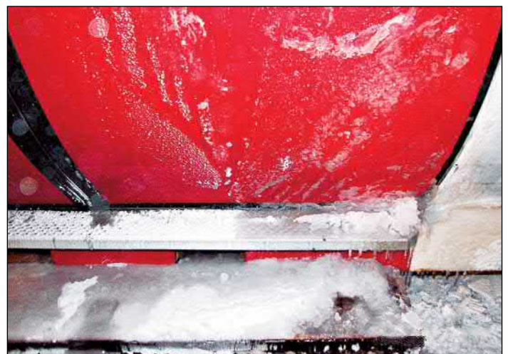
Photos 7: Movable door step with snow and ice build-up on a step.
