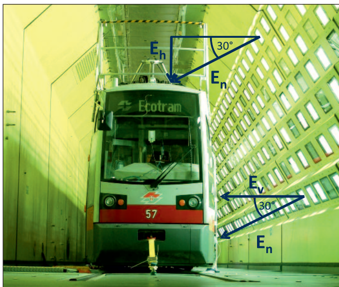
Figure 3: Correlation of equivalent E_n , vertical E_v and horizontal E_h solar radiation (intensity) in the climatic wind tunnel.
