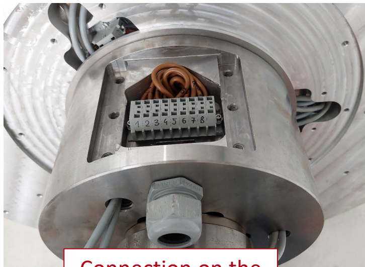
Connection on the shaft to the rotor
