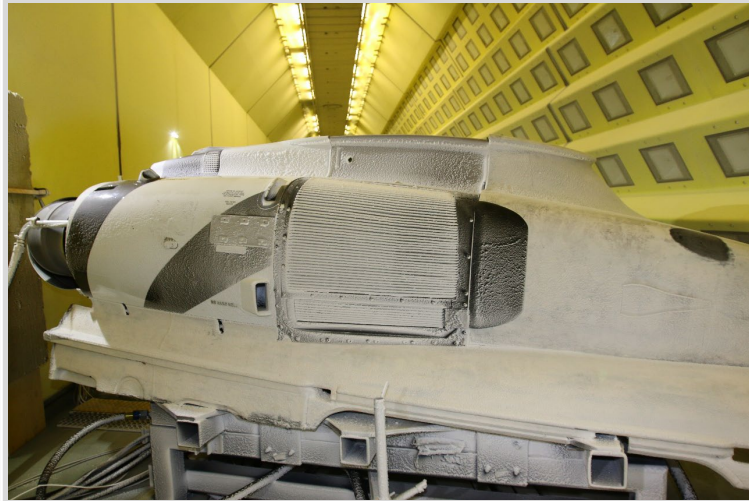
Exhaust gas system (air inlet filter with running engine)
